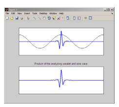
The product shown in the bottom pane closely resembles the analyzing wavelet. Integrating this product results in a CWT coefficient near zero.
