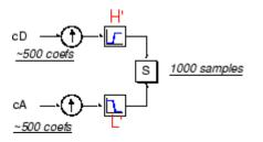
It is also possible to reconstruct the approximations and details themselves from their coefficient vectors. As an example, let's consider how we would reconstruct the first-level approximation A1 from the coefficient vector cA1.
