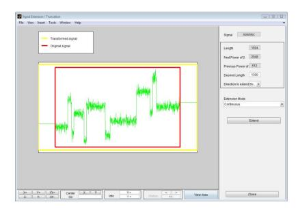
The signal is extended in both directions by replicating the first value to the left and the last value to the right, respectively.
