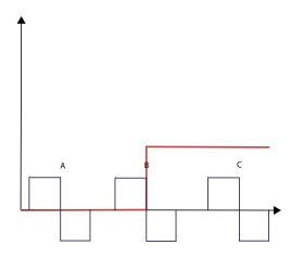
In the preceding figure, the red function is the shifted unit step function. The black functions labeled A, B, and C depict Haar wavelets at the same scale but different positions. You can see that the CWT coefficients around position A are zero. The signal is zero in that neighborhood and therefore the wavelet transform is also zero because any wavelet integrates to zero.
