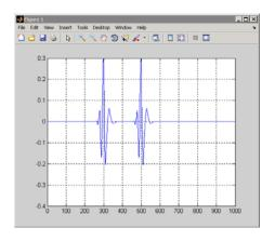
Next, look at the point 400 at scale 80. At scale 80, the cones of influence for both points 300 and 500 include the point 400. Even though the signal is zero at point 400, you obtain a nonzero CWT coefficient at that scale. The CWT coefficient is nonzero because the support of the wavelet has become sufficiently large at that scale to allow signal values 100 points above and below to affect the CWT coefficient. You can confirm this by entering:
