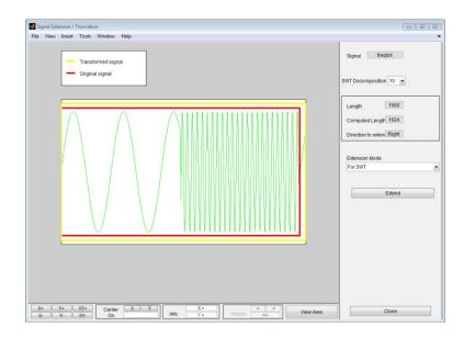
Since the signal is of length 1000 and the decomposition level needed for SWT is 10, the tool performs a minimal right periodic extension. The extended signal is of length 1024.
