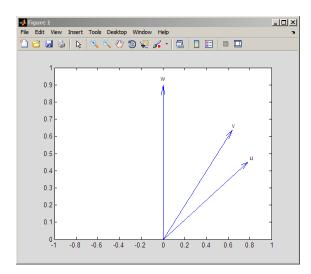
The inner products capture this geometric fact. Mathematically, the inner product of two vectors, u and v is equal to the product of their norms and the cosine of the angle,  $\theta$ , between them:
