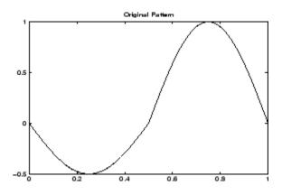
% To synthesize a new wavelet adapted to the given pattern, use % a least squares polynomial approximation of degree 6 with % constraints of continuity at the beginning and the end of the % pattern.
