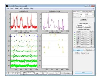
You can deselect the currently selected coefficients by double clicking each of them. Another way to select or deselect a set of coefficients is to use the selection box. Drag a rubber band box (hold down the left mouse button) over a portion of the coefficient axes (original or selected) containing all the currently selected coefficients. Click the **Unselect** button located on the right of the window. Click the **Apply** button. The tool displays the null signal again.
