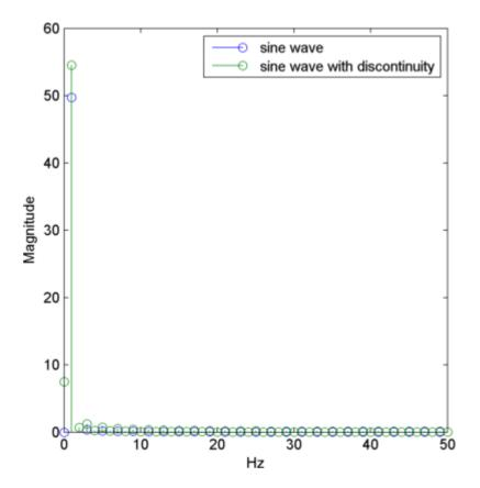
There is minimal difference in the magnitudes of the Fourier coefficients. Because the discrete Fourier basis vectors have support over the entire time interval, the discrete Fourier transform does not detect the discontinuity as efficiently as the wavelet transform.
