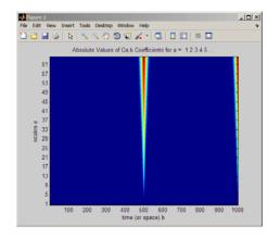
Similar to the shifted impulse example, the abrupt transition in the shifted step function results in large CWT coefficients at the discontinuity. The following figure illustrates why this occurs.
