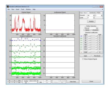
Select 16 coefficients individually by double clicking each of them using the left mouse button. The color of selected coefficients switches from green to yellow for the details and from blue to yellow for the approximation, which appear on the left of the window and appear in yellow on the middle part. Click the **Apply** button.
