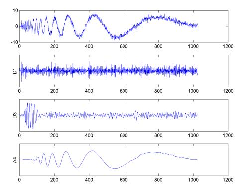
The wavelet and approximation coefficients at each level are equal in length to the input signal. The additive noise is almost entirely localized in the level one detail coefficients. The level 3 details coefficients captures the high-frequency oscillations at the beginning of the Doppler signal. The level 4 approximation coefficients are a lowpass approximation to the Doppler signal.
