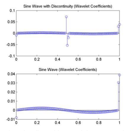
The wavelet coefficients of the two signals demonstrate a significant difference.
