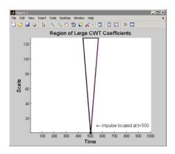
This region is referred to as the *cone of influence* of the point t=500 for the Haar wavelet. For a given point, the cone of influence shows you which CWT coefficients are affected by the signal value at that point.
