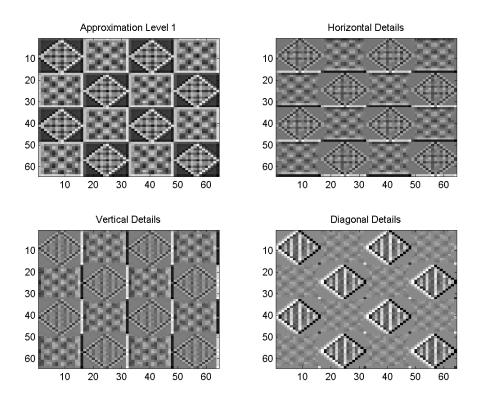
You see that the wavelet details are sensitive to particular orientations in the input image. The approximation coefficients are a lowpass approximation to the original image.
