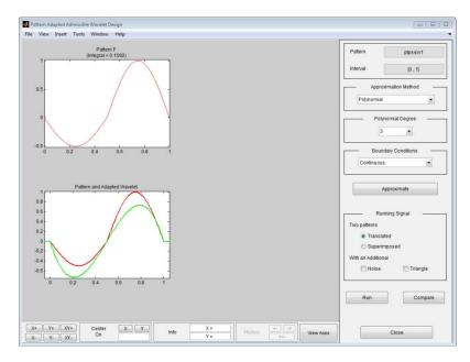
After a pause for computation, the tool displays the new wavelet in green superimposed with the original pattern in red.
