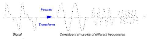
Because  $e^{j\omega t}$  is complex-valued,  $F(\omega)$  is, in general, complex-valued. If the signal contains significant oscillations at an angular frequency of  $\omega_0$ , the absolute value of  $F(\omega_0)$  will be large. By examining a plot of  $|F(\omega)|$  as a function of angular frequency, it is possible to determine what frequencies contribute most to the variability of f(t).
