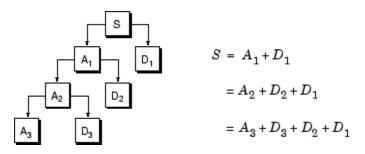
In wavelet packet analysis, the details as well as the approximations can be split.
