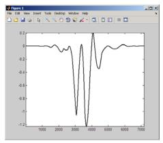
You can see that integrating over this product produces a negative CWT coefficient. That results because the wavelet is 1/2 cycle out of phase with the sine wave. The negative deflections of the wavelet approximately match the positive deflections of the sine wave. The positive deflections of the wavelet approximately match the negative deflections of the sinusoid.
