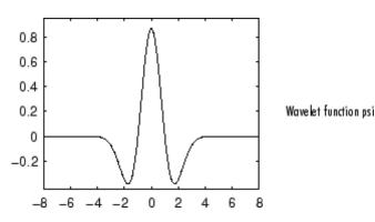
You can obtain a survey of the main properties of this family by typing waveinfo('mexh') from the MATLAB command line. See "Mexican Hat Wavelet: mexh" in the *Wavelet Toolbox User's Guide* for more information.
