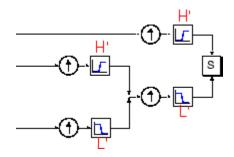
Where wavelet analysis involves filtering and downsampling, the wavelet reconstruction process consists of upsampling and filtering. Upsampling is the process of lengthening a signal component by inserting zeros between samples.
