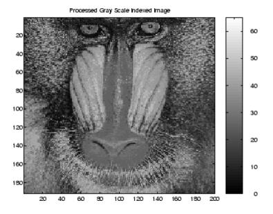
The color bar of the converted image is now linear and has a smooth transition from dark to light. The image is now suitable for wavelet decomposition.
