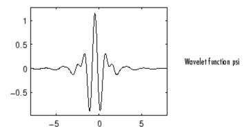
You can obtain a survey of the main properties of this family by typing waveinfo('meyer') from the MATLAB command line. See "Meyer Wavelet: meyr" in the *Wavelet Toolbox User's Guide* for more detail.
