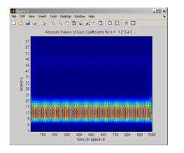
Note that the CWT coefficients are large in absolute value around scales 9 to 21. You can find the pseudo-frequencies corresponding to these scales using the command:
