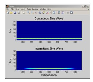
By using the STFT, you can see that the intermittent sine wave begins near 250 msec and ends around 750 msec. Additionally, you can see that the signal's energy is concentrated around 20 Hz.
