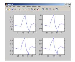
The curve begins to look progressively more like the db2 wavelet. This means that the wavelet's shape is determined entirely by the coefficients of the reconstruction filters.
