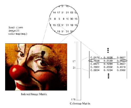
Outside MATLAB, indexed images with n colors often contain values from 0 to n–1. These values are indices into a colormap with 0 as its first index. Since MATLAB matrices start with index 1, you must increment each value in the image, or *shift up* the image, to create an image that you can manipulate with toolbox functions.
