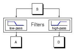
The original signal, S, passes through two complementary filters and emerges as two signals.
