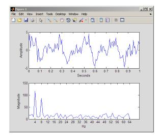
Viewed as a time signal, it is difficult to determine what significant oscillations are present in the data. However, looking at the absolute value of the Fourier transform coefficients as function of frequency, the dominant oscillations at 4 and 8 Hz are easy to detect.
