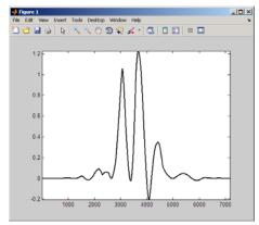
You can see that integrating over this product produces a positive CWT coefficient. That results because the oscillation in the wavelet approximately matches a period of the sine wave. The wavelet is *in phase* with the sine wave. The negative deflections of the wavelet approximately match the negative deflections of the sine wave. The same is true of the positive deflections of both the wavelet and sinusoid.
