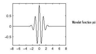
You can obtain a survey of the main properties of this family by typing waveinfo('morl') from the MATLAB command line. See "Morlet Wavelet: morl" in the *Wavelet Toolbox User's Guide* for more detail.
