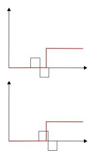
In the top figure, the wavelet has just begun to overlap with the unity portion of the unit step. In this case, the CWT coefficients are negative, but not as large in absolute value as those obtained at position B. In the bottom figure, the wavelet has shifted past position B and the positive deflection of the wavelet begins to contribute to the integral. The CWT coefficients are still negative, but not as large in absolute value as those obtained at position B.
